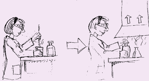
Figure 4: Installing a ventilation system to remove unwanted fumes
