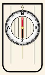
Basic compass with no declination adjustment. True north and magnetic north are are the same in this example.
