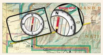
Now turn the azimuth ring so the orienting arrow and the compass needle are aligned. The value that the index pointer shows is your bearing to that location (75° East Northeast in this example).
