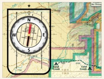
Set the compass's declination for your area. Note that the magnetic north and declination are aligned, (10.5° E in this example), while true north is at the top of the page and map.
